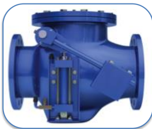
Slow down the check valve closure. It should take 5 seconds per inch diameter, or more.
