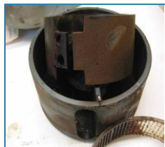
lime scale in a PD meter
