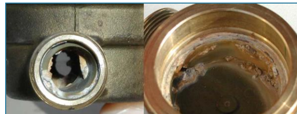
Lime scale built-up in the single jet water meter housing
