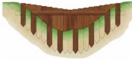
Figure 11 Log Check Dam
