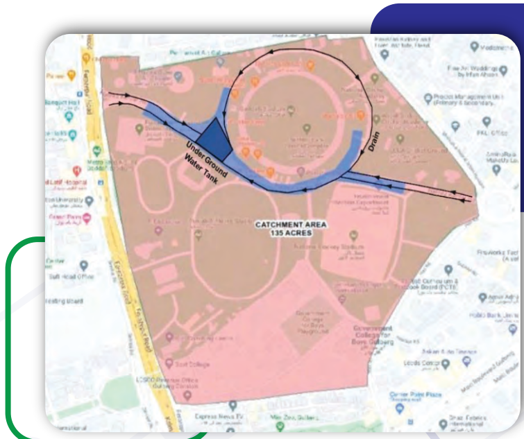
Fig 9: Scheme of Stormwater Storage Tank and drains to eliminate urban flooding at Nishtar Park Stadium Lahore.
